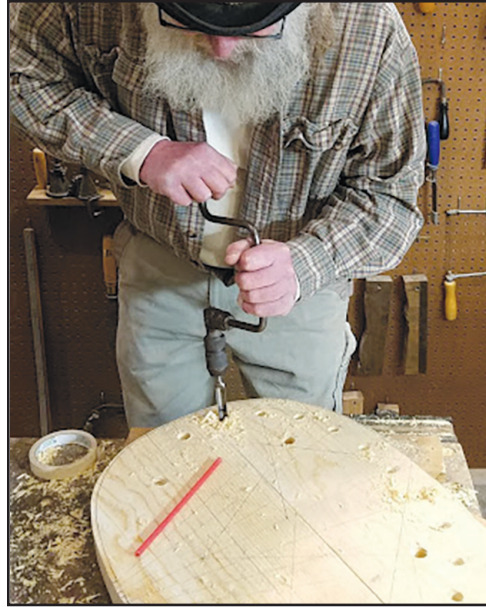
Using brace bit to drill holes for the legs.
