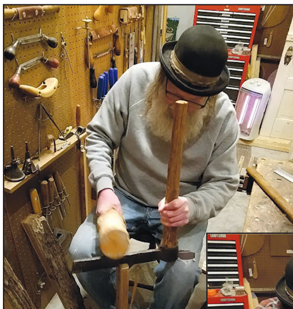
Using froe to chop parts for spindles.
