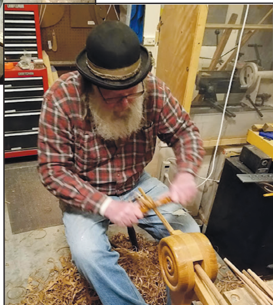
Using shaving post to carve spindles.
